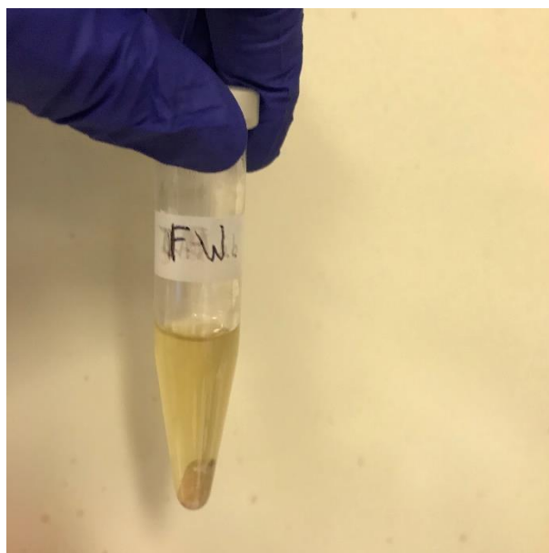
Figure 4 – The sample containing washed fleece microfibres after irradiation.
